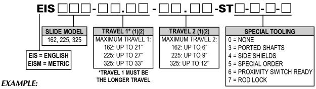
To order an EIS225 Series Slide, with travel 1 of 6.00 inches and travel 2 of 3.00 inches and ported shafts:
