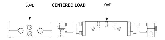
**MAXIMUM DEFLECTION** =  $\frac{\text{LeA}^2(3\text{L}-4\text{A})}{\text{C}}$ Le = 1/2 (WI + Ws)
